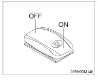
(1) This switch turns ON the rotary light on the cab.
