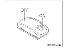
(1) This switch is used to operate head lamps. Press this switch to turn on head lamps.
